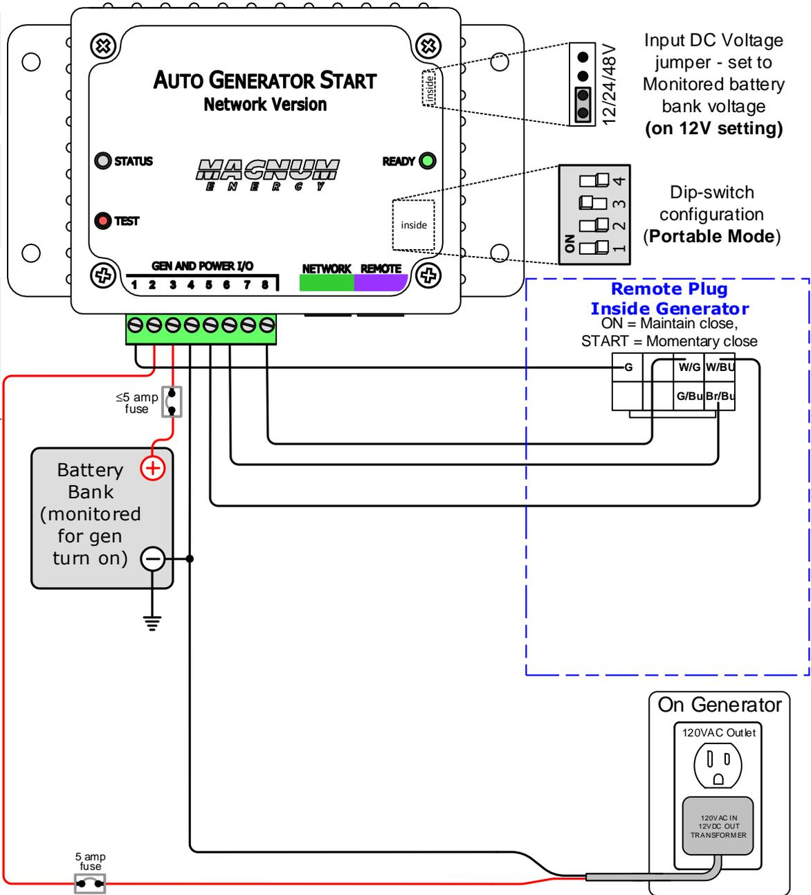
Gen Run Signal (input to pin 2 must be 10 to 40 DC volts only while generator is running); can be the generator hour-meter, a 12vdc pilot/run light, or see Alternative Options in the AGS Manual
