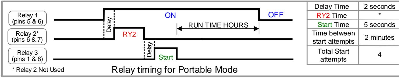
Magnum Energy, Inc. provides this diagram to assist in the installation of the Auto-Generator Start controller. Since the use of this diagram and the conditions or methods of installation, operation and use are beyond the control of Magnum Energy, Inc., we do not assume responsibility and expressly disclaim liability for loss, damage or expense arising out of the installation, operation and use of this unit.
