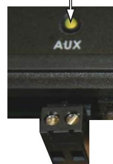
Aux Relay LED Indicator
